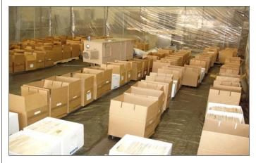
Dehumidification chamber with fans and dehumidifiers to dry out the boxes and folders.
