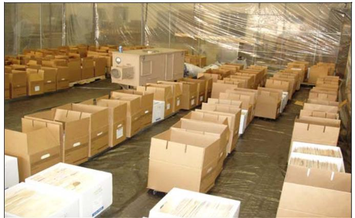
*Dehumidification chamber with fans and dehumidifiers to dry out the boxes and folders.*
